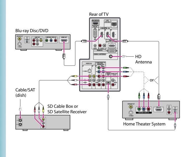
• Your TV is equipped with four HDMI inputs and two component inputs. Connect your incoming signal source (HD Cable Box, HD Satellite Receiver, or DVD) with
