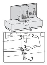
10 For models with swivel stand (KDL-32T30xx, KDL-40T30xx) do not tense the support belt.
