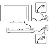
**1** Connect the display unit and media receiver unit to wall
