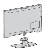
**3** Fix the stand to the TV using the supplied screws.
