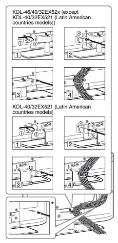
\* When installing on the wall, attach the cable holder under the terminals.
