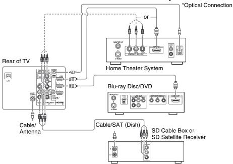
\* The optical connection is only needed for A/V receivers that do not support ARC (Audio Return Channel).
