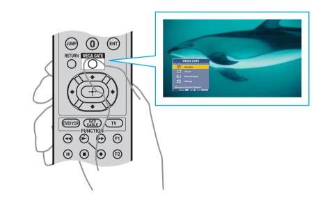
To adjust Settings related to Video, Audio, Screen, Channel, Parent (V-chip), Clock/ Timers or to set up certain features on your TV, press then select "Settings" on the WEGA GATE control panel.
