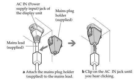
To unplug the mains lead pull down the mains plug holder by pushing in both sides of the holder than any lead of t sides of the holder, then pull out the plug.
