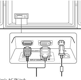
**2** Secure the mains plug to the display's AC IN jack.
