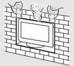
Leave some space around the TV set as shown below. Otherwise, air-circulation may be inadequate and cause overheating, which may cause a fire or damage to the TV set.
