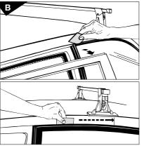
GB Open the front door and insert the plastic card between the roof and the rubberweatherstrip as shown in Fig B. Carefully draw the card backwards until it iscentred on the position for the rear load
