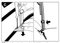
GB Use the plastic card to fold the rubber weatherstrip outwards, and push the bracket downwards between the roof and the card. Note that the bracket should be pushed downwards until it is touching the roof. Remove the plastic card when the bracket has been fitted.
