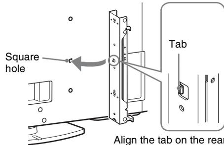
Align the tab on the rear of the Mounting Hook with the square hole on the rear of the TV as illustrated.
