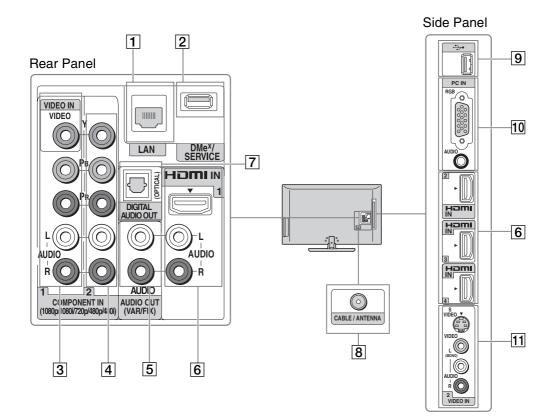
• An HDMI or Component video ( $YP_BP_R$ ) connection is required to view 480i, 480p, 720p, 1080i and 1080p video formats. The 1080/24p video format is available only with HDMI connection. This TV displays all video input signals in a resolution of 1,920 dots × 1,080 lines.
