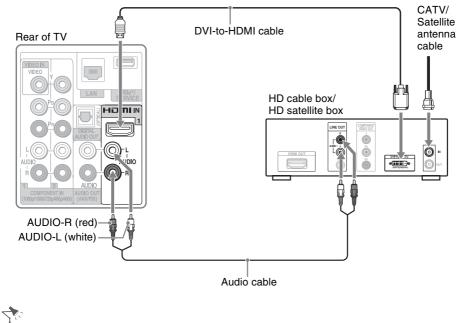
• If your equipment has a DVI output and not an HDMI output, connect the DVI output to the HDMI IN 1 (with DVI-to-HDMI cable or adapter) and connect the audio output to the AUDIO IN (L/R) of HDMI IN 1.
