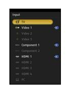
The TV will automatically detect the connected equipment. Shown here with equipment connected to Video 1, Component 1 and HDMI 1.
