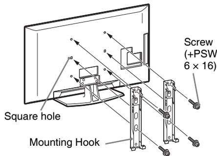
Sufficient expertise is required for installing this product, especially to determine the strength of the wall for withstanding the TV's weight. Be sure to entrust the attachment of this product to the wall to Sony dealers or licensed contractors and pay adequate attention to safety during the installation. Sony is not liable for any damage or injury caused by mishandling or improper installation.
