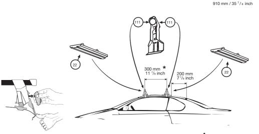
Screw the load carrier into position alternating between the feet, and maintaining constant pressure on the bracket.
