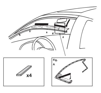
Undo the 6 screws that hold the trim. Place the shim strip in the bottom of the trim as shown in figure A. Insert the strip so that it fills up the space between the trim and the inner raingutter. Refit the braced trim.
