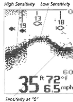
To adjust Sensitivity, press MENU repeatedly until the Sensitivity heading is displayed. When the Sensitivity menu appears, use the UP ARROW to increase the Sensitivity, or the DOWN ARROW to reduce the sensitivity. To sequence through the available settings, press and hold either ARROW button. Release the button at the setting you want to change.
