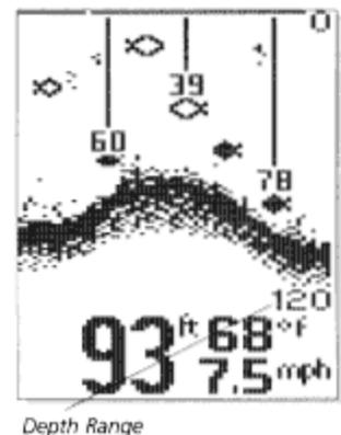
Using manual Depth Range control, you can view sonar information from the area near the surface in great detail.
