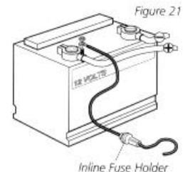
The Power can be connected to the boat's electrical system at two places: a fuse panel, usually located near the console, or directly to the battery.
