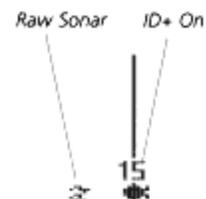
Increasing the value to a number greater than zero shows more fish symbols on-screen. In this case smaller sonar returns will be depicted as fish symbols. This is useful for identifying many smaller sonar returns (such as baitfish) as fish symbols.
