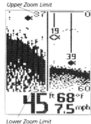
Automatic Zoom is especially helpful when looking for structure or bottom detail. The Automatic Zoom keeps the bottom in view even in quickly changing terrain, but is most useful in flatter areas without considerable depth variation. Manual Zoom provides detailed information of any area from the surface to the bottom. In manual Zoom, the Zoom range does not move as the terrain changes.
