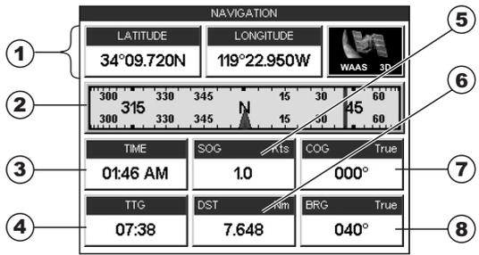
Figure 12.2a - Navigation Data page with Compass Tape
