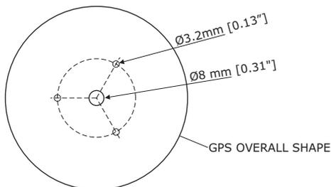
Figure 2.3.0a - Installing the External GPS Antenna (II)
