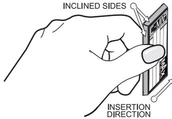
Figure 5.0 - Inserting C-CARD
