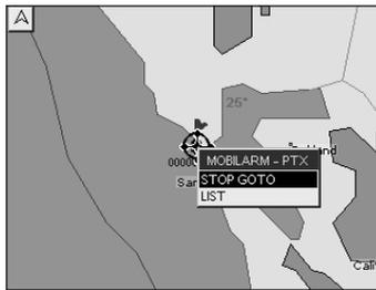
Figure 16.4.1b - Example of Stop Goto PTX on CP180
