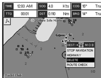
Figure 8.0 - Deleting MOB point on CPF180i
