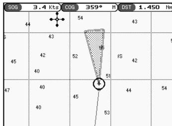
Figure 13.3 - Grounding Alarm
