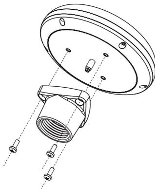
Figure 2.3.0 - Installing the External GPS Antenna (I)
