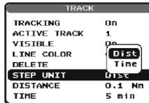
Figure 10 - Distance Units and Time Units
