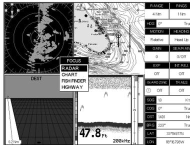
Figure 17.2.4.2 - Example of Combo Page with **[Focus]** shown
