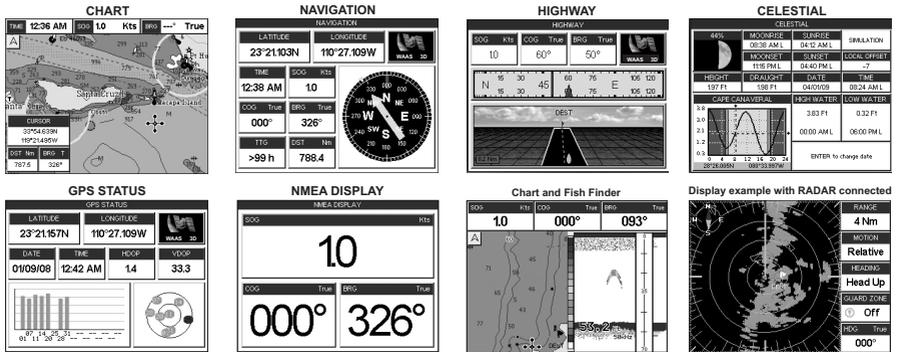
Figure 12 - Example of screen display pages for CPF300i
