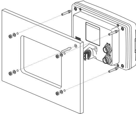
Figure 2.2 - Example of Flush installation CPF180i
