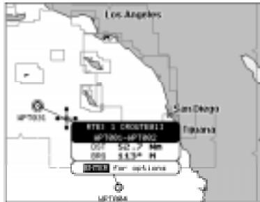
Figure 3.8.3 - Placing Waypoint between two existing ones (I)
