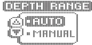
The Tracker unit automatically adjusts the depth range depending on the depth of the water. The unit tries to maintain the bottom depiction about  $\frac{2}{3}$  down the total range (for example, in 20' (6m) of water, the 0-30' (0-10m) range would be selected). This provides the best display resolution and therefore the best target separation possible.
