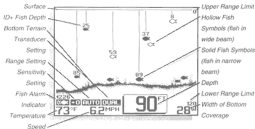
The Wide Vision allows you a number of ways to display sonar information. Some features are used in conjunction with special accessories such as the Boat Speed and Water Temperature gauge, or "Wide Side" side looking transducer.
