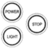
POWER, as previously discussed, powers the Wide Vision for normal operation. Also, if the unit is powered off, press and hold POWER until you hear a continuous "chirp" to enable simulator operation as discussed in "Simulator Operation." Pressing POWER when the unit is in normal or simulator operation will power the unit off.
