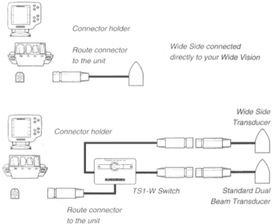
Also, several kits are available that include a Wide Side transducer with a switch or an additional mounting system. (See Section One, Available Accessories)
