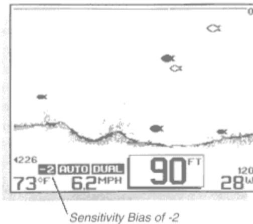
Another use of the Sensitivity menu is to select the bottom representation. The Wide Vision normally displays a variable Structure ID bottom, which can allow experienced users to determine the texture or relative hardness of the bottom. For simplicity, you can select a black bottom using the ENTER button. This blackens in the display below the bottom for easiest recognition of the bottom location, even from a great distance.
