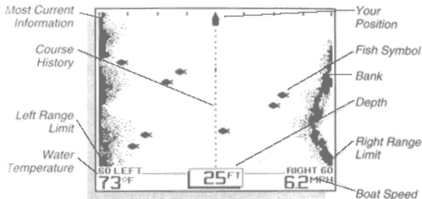
Experiment with the Wide Side transducer while operating it in a familiar area and learn how to make maximum use of the information displayed. Remember, if you are using a trolling motor mount, the information displayed is controlled by the direction the trolling motor is pointing, not necessarily the direction the boat is travelling.
