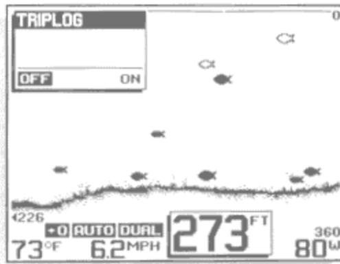
The TripLog can be reset at any time by pressing STOP. Press ENTER to return to the normal screen.
