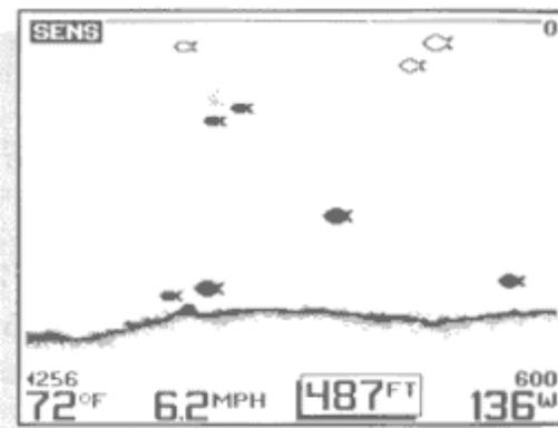
The base screen layout is modified to maximize the display for terrain and target presentation. To accomplish this, symbols such as Sensitivity setting, and Fish Alarm indicators, are removed.
