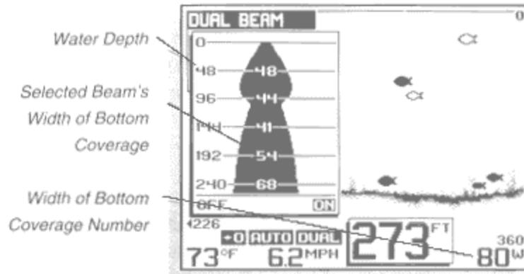
The options in the Transducer menu are "Dual", which uses both transducer elements for transmitting and receiving the sonar signals, "Narrow" which selects ments available in the Transducer menu will be "Left", "Right", and "Both". More information about these options is discussed in "Wide Side Operation".
