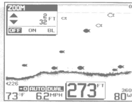
Another form of range control is Zoom. Zoom allows selection of various ranges for full screen viewing, while maintaining a view of the full range. By using the display to view a smaller area, the effective display resolution is increased, and the units ability to separate targets close together is enhanced.
