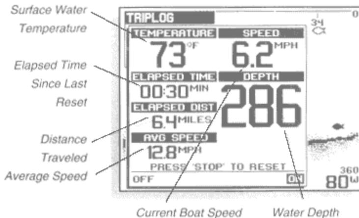
Note: The Temperature|Speed accessory must be connected for TripLog to work.
