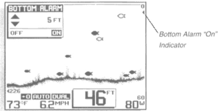
To disable the alarm, either move to deeper water, or select the Bottom Alarm menu, and press ENTER to turn the alarm off.
