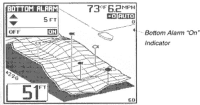
To disable the alarm, either move to deeper water, or select the Bottom Alarm menu, and press ENTER to turn the alarm off.
