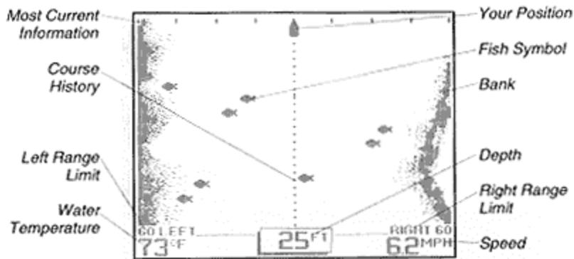
When you exit the "System Options" menu, the view you will see on-screen is shown above. Viewing both left and right sides simultaneously gives you an excellent tool when searching for bait fish or following a creek bed, however greater display resolution can be achieved by viewing only one side.
