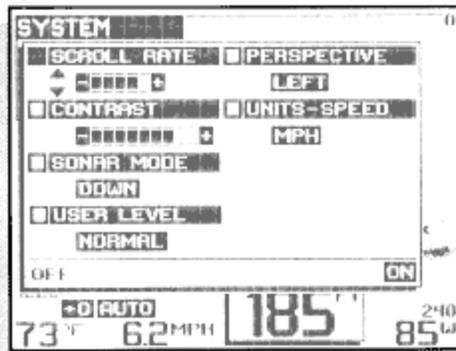
User Level is used to select Normal or Advanced operation. Advanced mode performs several functions which will benefit the experienced user. Icons are not shown and numerical data is smaller to allow more of the display to be used for the picture of the bottom. Several other changes in operation occur which are designed to increase the speed of adjustments, and maximize the graphic use of the display. Refer to "Advanced Operation" for more detailed information.
