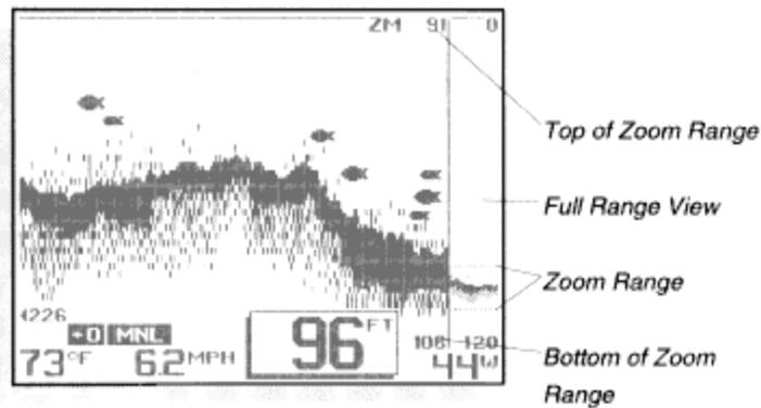
To enable Zoom, adjust the horizontal lines to the depth of the zoom range using the UP and DOWN arrow buttons, then enable Zoom using the ENTER button.
