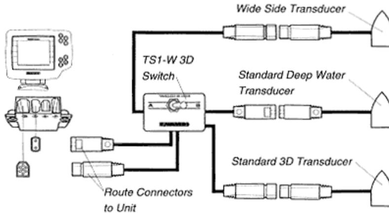
When the Wide Side transducer is connected directly to your unit, or selected using a transducer switch, the unit setup must be changed to correspond with the type of transducer being used. This adjustment is made through the "System Options" menu. Use the MENU button to select the "System Options" menu and press ENTER. Press MENU until the "sonar mode" option is highlighted. Press UP or DOWN until "side" is displayed. Press ENTER when the selection is correct.
