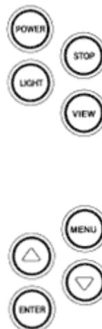
MENU brings a menu on-screen for adjustment, or if a menu is already present, the next menu in sequence will appear. Menus will go off-screen and normal operation will resume after a short period of time. If you wish to keep the menu on-screen for an extended period of time, press STOP.
