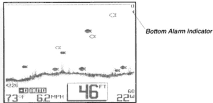
The Fish Alarm alerts you to the presence of fish, or other targets not attached to the bottom, in the water beneath your boat. The Fish Alarm has 3 different settings which correspond to the 3 different size fish targets shown on-screen.
