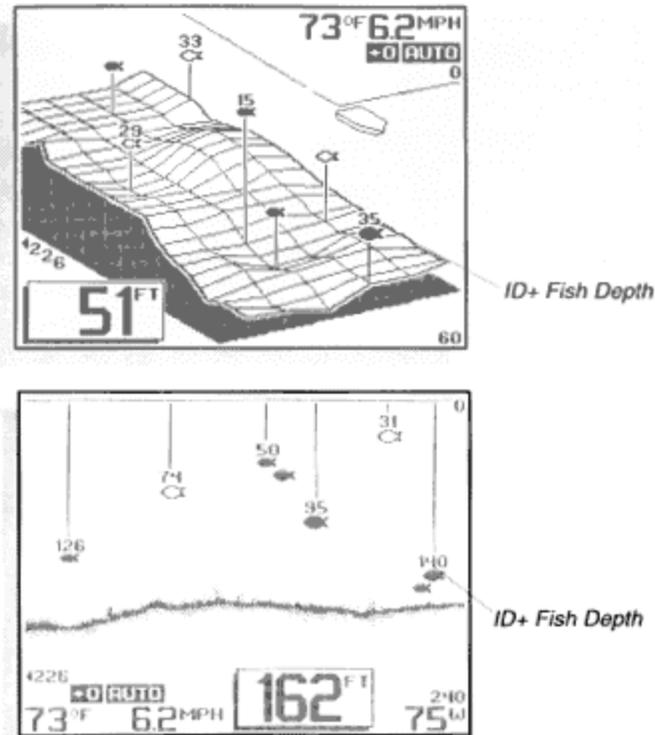
"ID+", the default setting, provides more information about the location of the target by attaching depth "strings" showing the digital depth of the target. When there are numerous targets on-screen, not every target depth is shown, to avoid excessive clutter on-screen.
