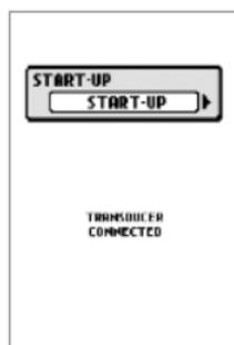
When the PiranhaMAX™ powers on, the Start-Up menu temporarily appears. From this menu, select either Start-Up, Simulator, or SetUp.
