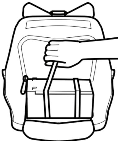
3. Pull the two battery tie-down straps over the top of the battery and connect both ends of each strap over the top, making sure that the straps are pulled tight around the battery and that the battery is seated securely in the battery well.
