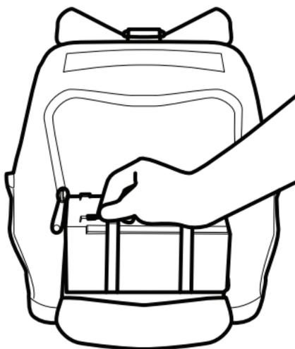
4. Make sure the back battery door and side pockets are zipped, but leave the front of the bag unzipped for easy access during installation.
