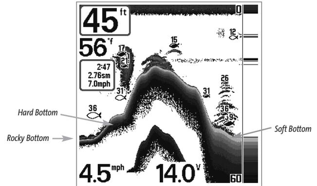
The sonar returns from the bottom, structure and fish can be represented as either **Inverse** (default), **Whiteline®**, **Structure ID®**, or **Bottom Black**. See *Sonar X-Press™ Menu: Bottom View* for details on how to set the bottom view.
