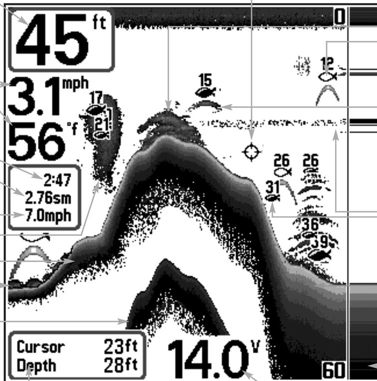
**Cursor Dialog Box** - indicates cursor depth on the display and the depth of the bottom directly below the cursor.
