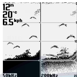
Split window 50kHz/200kHz, shown with metric depth, °C and kph digital readouts available on international models.
