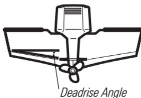
**NOTE:** The hydrodynamic shape of your transducer allows it to point straight down without deadrise adjustment.
