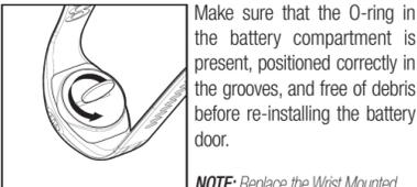
Make sure that the O-ring in the battery compartment is present, positioned correctly in the grooves, and free of debris before re-installing the battery door.
