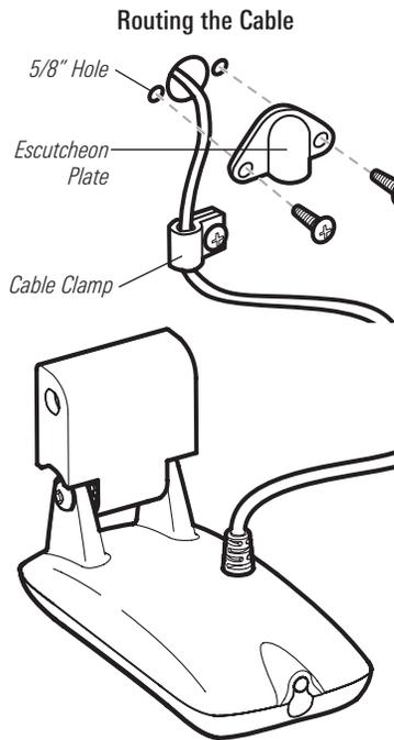
3. Place the escutcheon plate over the cable hole and use it as a guide to mark the two escutcheon plate mounting holes. Remove the plate, drill two 9/64" (3.5 mm) holes, then fill both holes with marine-grade silicone sealant. Place the escutcheon plate over the cable hole and attach with two #8 x 5/8" (16 mm) wood screws.
