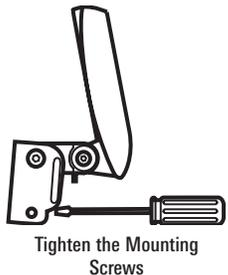
3. Adjust the height of the assembly so the face of the transducer is 1/8" (3 mm) to 1/4" (6 mm) beneath the bottom of the transom, and fully tighten the three mounting screws.
