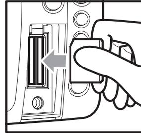
Inserting an MMC/SD
