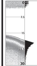
The **Wide RTS® Window** indicates the sonar intensity through the use of a bar graph. The length of the plotted return provides an indication of whether the return is weak or strong. The depth of the sonar return is indicated by the vertical placement of the return on the display depth scale.
