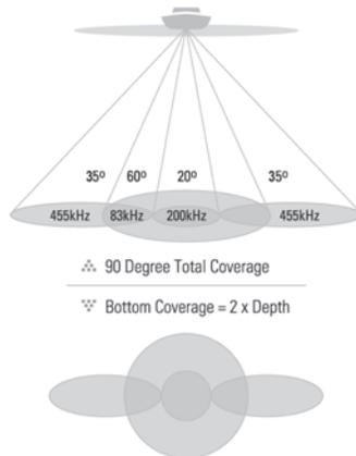
Your 900 Series™ 997c Combo supports the optional-purchase QuadraBeam PLUS™ transducer. QuadraBeam PLUS™ sonar provides an extremely wide (90°) area of coverage. QuadraBeam PLUS™ starts with two fan-shaped 35° 455 kHz Side Structure locating sonar beams to spot fish, bait and structure to the left and right of the boat over an area of the bottom that's always equal to twice your depth.
