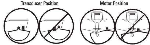
The Side Imaging transducer has some special requirements because of its side viewing capabilities:
