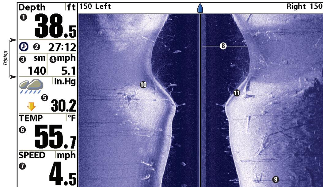
**8** The **water column** shows the relative depth of the water under the boat at a given time. Variations in the width of the water column show variations in the distance to the bottom as the boat passes over.
