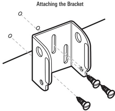
5. Align the metal mounting bracket with the mounting holes. The center slot should be above the two outer slots. (This bracket and all other hardware supplied is top quality stainless steel for maximum strength and corrosion protection.) Insert the three 1" (25 mm) flat head wood screws into the drilled holes, but do not completely tighten.
