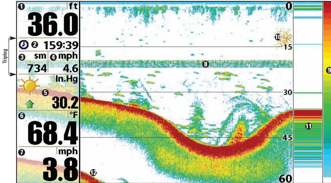
**7 Speed** - if a Speed accessory or GPS Receiver is attached, the 900 Series™ can display the speed of the boat, and can keep a triplog of nautical or statute miles traveled.
