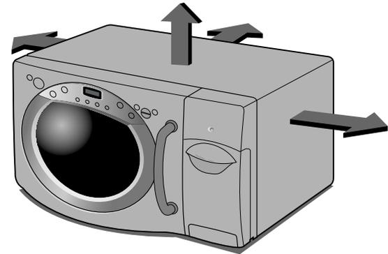
The right side in which has exhaust outlet must be at 10 cm from wall or something to block.
