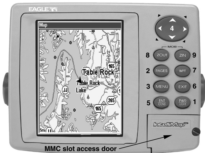
IntelliMap 502C GPS unit, front view, showing Map Page, keyboard and access door for the MMC slot.
