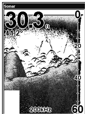
Full Sonar Chart. The Overlay Data (depth and water temperature) are set to different text sizes.
