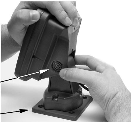
**Adjust viewing angle: use one hand to press and release the spring-loaded ratchets while you move the unit with the other hand. An optional GBSA-3 swivel base is shown with the quick release bracket.**
