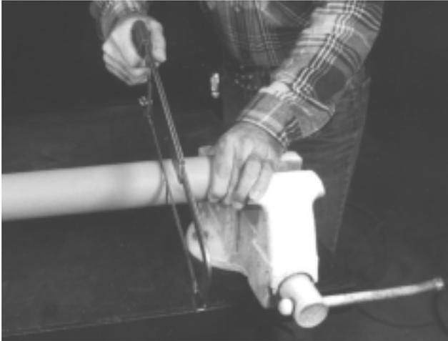
H. Using cut off section of shield as a guide, cut shaft the same amount. (Figure 2-4)
