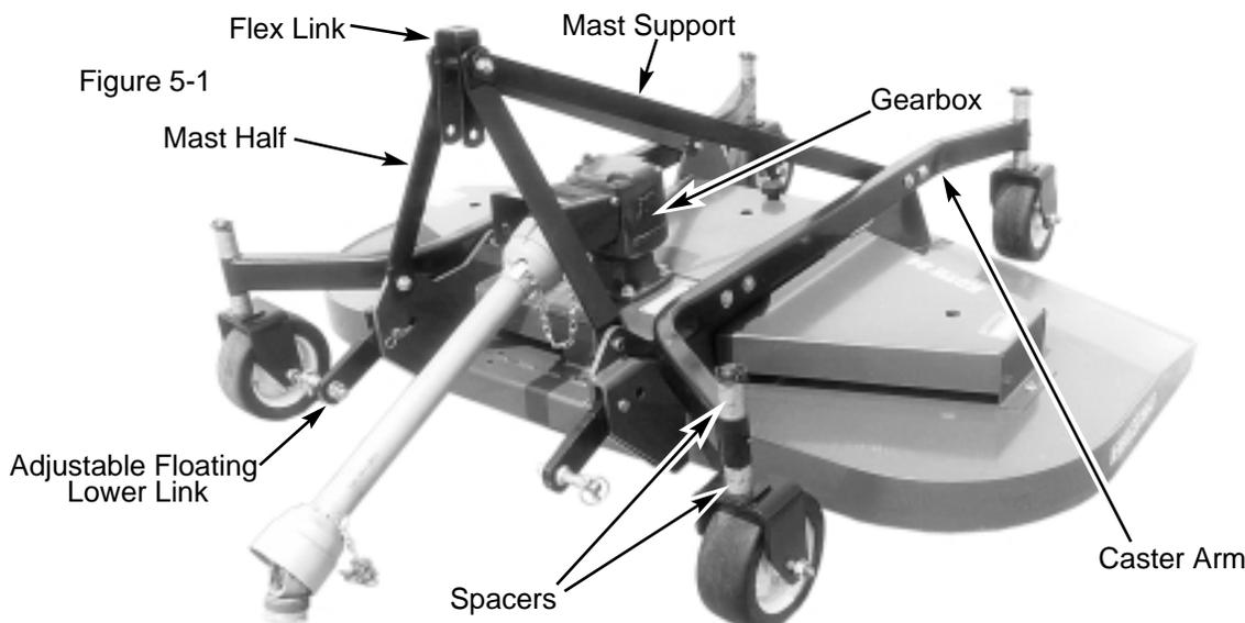
E. Fasten mast supports and upper flex link to mast halves using 5/8" x 5-1/2" bolt, pivot tube, lockwasher and locknut.
