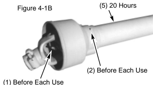
line and shields are securely connected. Make certain PTO shielding is in good condition.
