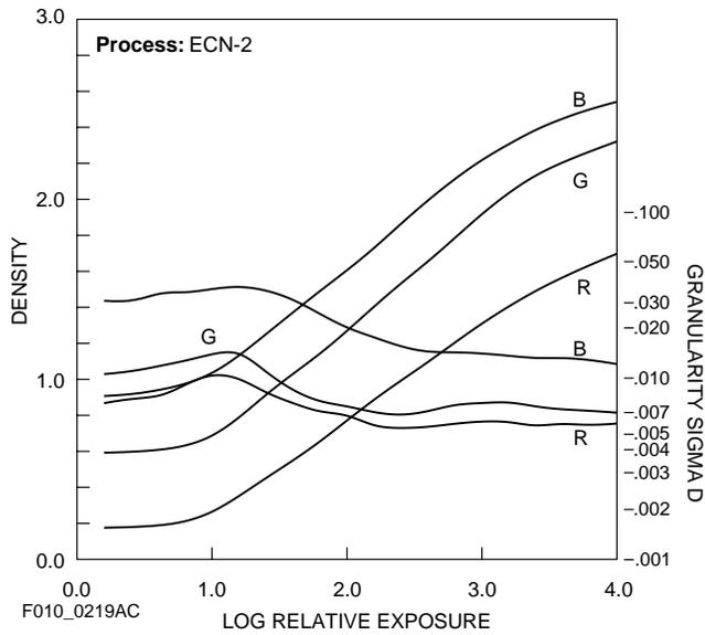
To find the rms Granularity value for a given density, find the density on the left vertical scale and follow horizontally to the characteristic curve and then go vertically (up or down) to the granularity curve. At that point, follow horizontally to the Granularity Sigma D scale on the right. Read the number and multiply by 1000 for the rms value.
