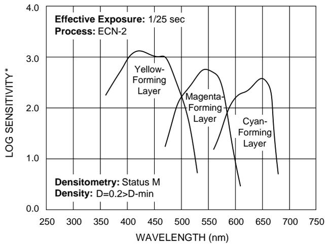
\*Sensitivity = reciprocal of exposure (erg/cm<sup>2</sup>) required to produce specified density
