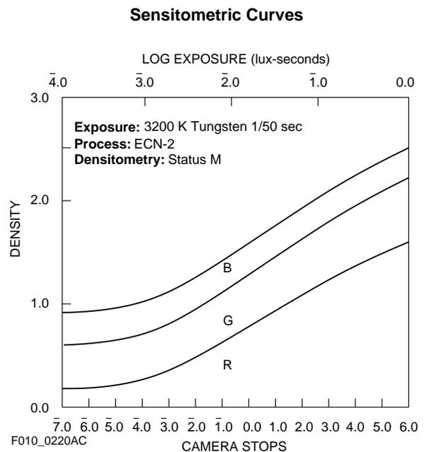
The curves describe this film's response to red, green, and blue light. Sensitometric curves determine the change in density on the film for a given change in log exposure.<sup>4</sup>
