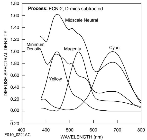
These curves depict the spectral absorptions of the dyes formed when the film is processed. They are useful for adjusting or optimizing any device that scans or prints the film.
