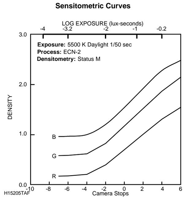
The curves describe this film's response to red, green, and blue light. Sensitometric curves determine the change in density on the film for a given change in log exposure.<sup>3</sup>
