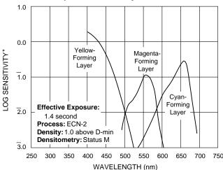
\*Sensitivity = reciprocal of exposure (ergs/cm<sup>2</sup>) required to produce specified density
