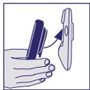
Place the Twin-Phone in the hang-up cup of the Bury hands-free car kit in order to enable power supply to reach the device. If such supply is continuous, the device will immediately switch on. If not, the system will be activated upon ignition and/or starting the engine.
