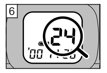
Check the exposure counter (telling the number of exposures remaining).
