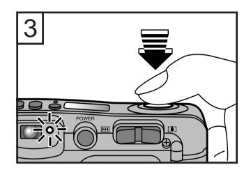
With the AF frame positioned over the subject, press down the shutter release button halfway to set the auto-focus lock.
