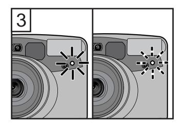
After the self-timer lamp remains lit for about 7 seconds, it blinks for about 3 seconds, and then the shutter is released. When taking consecutive exposures, the shutter is released the set number of times at an interval of between 3 and 6 seconds.
