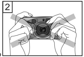
Make sure that nothing is in front of the lens, the flash, the autofocus windows or the automatic exposure light sensor.
