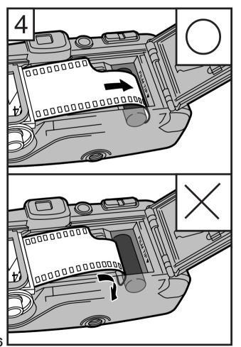
Make sure the end of the film is threaded onto the spool.
