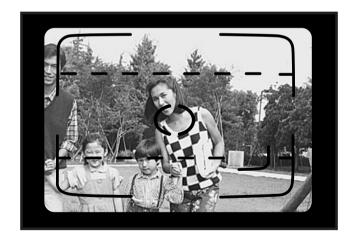
2. Move the camera slightly and.... aim the Autofocus Spot so that it covers some part of your subject, then press the Shutter Release about halfway down (to lock the focus) and make sure the Autofocus Lamp (focusing completed signal) has turned on.
