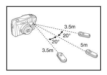
**4. Effective switch range**The effective range of the Remote Control Switch is about five meters when held directly in front of the camera, and up to 3.5 meters when aimed at the camera at a 20° angle from all sides (left, right, above, and below).
