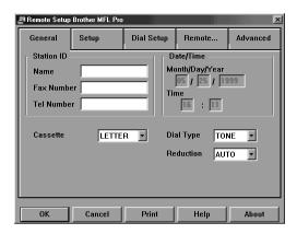
When the MFC Remote Setup dialog box first appears, the settings on your MFC 4300 will be downloaded to your PC and displayed on your computer screen. Instead of programming directly on your MFC control panel, fill in the information in the **General**, **Setup**, **Dial Setup**, **Remote** and **Advanced** tabs. After you enter setup information and change default settings, you can upload your changes directly to the MFC.
