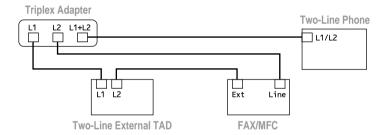
You can keep two-line telephones on other wall outlets as always. There are two ways to add a two-line telephone to the MFC's wall outlet. You can plug the telephone line cord from the two-line telephone into the L1+L2 jack of the triplex adapter. Or, you can plug the two-line telephone into the TEL jack of the two-line TAD.
