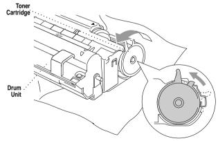
3 Remove the old toner cartridge from the drum unit by gently pulling it out.
