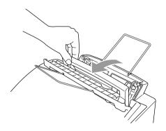
2 Fan the paper well. Load the paper, making sure the print side is toward the fax machine and the paper level is stacked below the paper mark. The feeder can hold up to 200 sheets of paper, or up to 10 envelopes.
