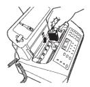
Pull the cartridge towards the front of the machine until you hear it click into position.
