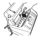
Use a slightly damp cloth to clean the electrical contacts taking care not to touch the nozzles.
