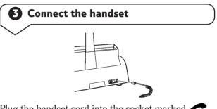
Plug the handset cord into the socket marked *f* at the back of the machine.
