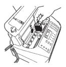
7 Pull the assembly towards the front of the machine until you hear it click into position.
