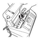
4 Remove the new printhead assembly from its packaging. Holding it by the finger grip, peel the protective film from the print nozzles.
