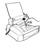
Remove the print cartridge from its packaging. Holding it by the finger grip, peel the protective film from the print nozzles.
