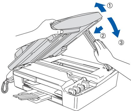
The machine will clean the ink tube system for use for the first time. This process will occur only once, the first time ink cartridges are installed. The cleaning process will last approximately four minutes.
