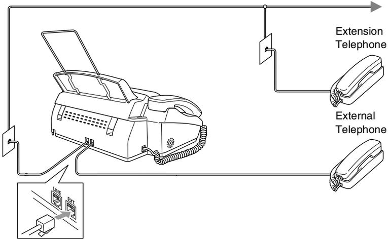
Whenever this external phone (or TAD) is in use, the screen displays **EXT. TEL IN USE**, and, if the fax handset is lifted, an alarm sounds.
