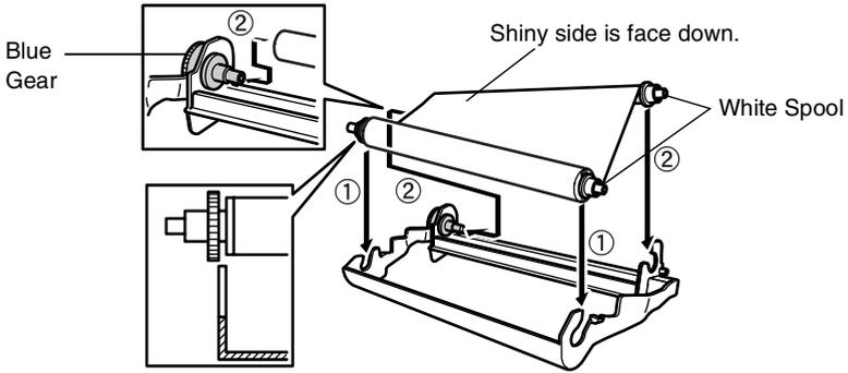
**7** Turn the upper right white spool *clockwise* to tighten the ribbon, as shown.
