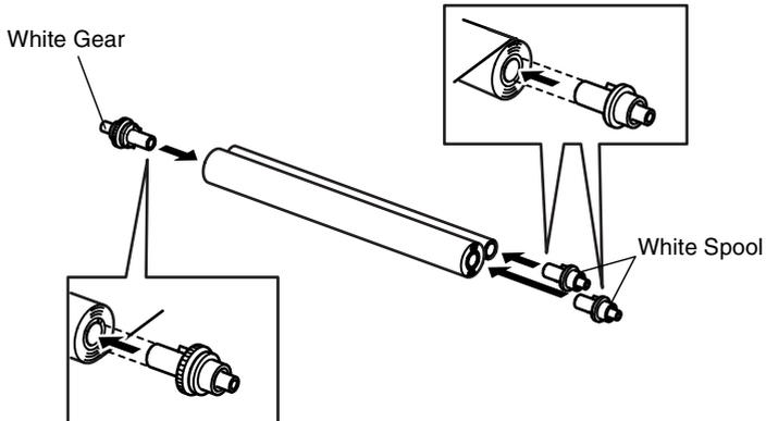
**6** Install the new ribbon in the cartridge:
