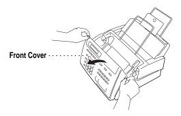
2 Open the top cover, pressing the blue levers on both sides of the top cover.
