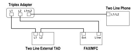
You can keep two-line telephones on other wall outlets as always. There are two ways to add a two-line telephone to the FAX/MFC's wall outlet. You can plug the telephone line cord from the two-line telephone into the L1+L2 jack of the triplex adapter. Or, you can plug the two-line telephone into the TEL jack of the two-line TAD.
