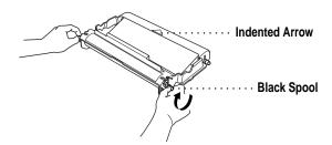
**5** Install the printing cartridge by inserting the indented  $\triangleq$  first and placing the cartridge into its four holders.
