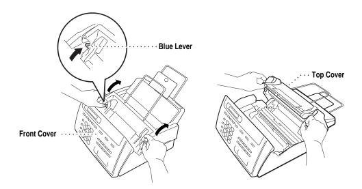
4 Pull the jammed paper gently from the paper feeder toward the back of the FAX/MFC. If the paper remains jammed, then pull it toward the front of the machine.
