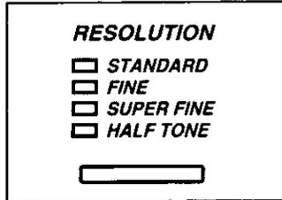
**STANDARD** is suitable for printed or typewritten originals with normal-sized characters.
