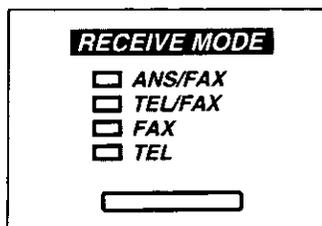
Press the **RECEIVE MODE** button to select the desired receiving mode.
