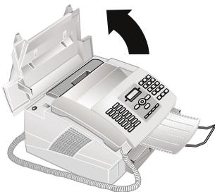
**2** Remove the old toner cartridge, by gripping it at the recess in the middle and pulling it upward.
