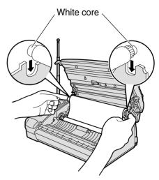
**5** If the ink film is slack, tighten it by winding the "T" shaped gear.
