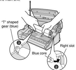
4 Insert the white core into the slots shown in the picture below.
