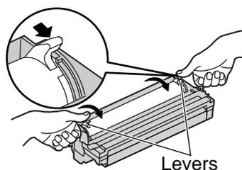
**11** The toner cartridge is installed when the triangles match.
