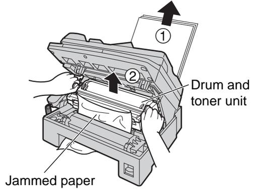
Remove the jammed paper from fuser unit by pulling it upwards carefully.
