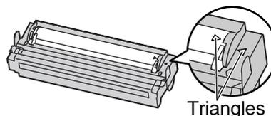
**12** Install the drum and toner unit by holding the tabs.
