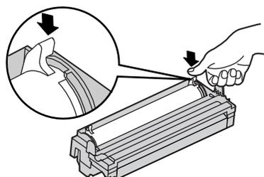
**6** Turn the two levers on the toner cartridge with firm pressure.
