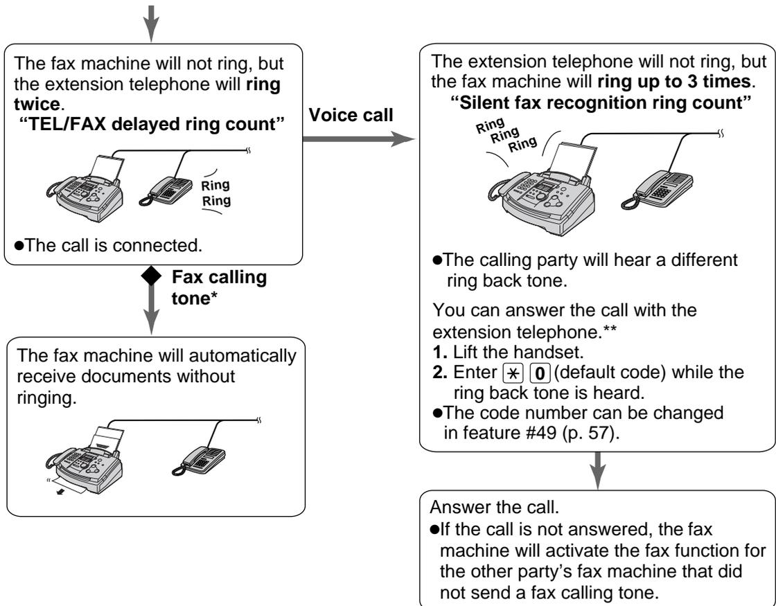
\* A fax calling tone is automatically generated by the sending fax machine. Some fax machines do not have this capability.
