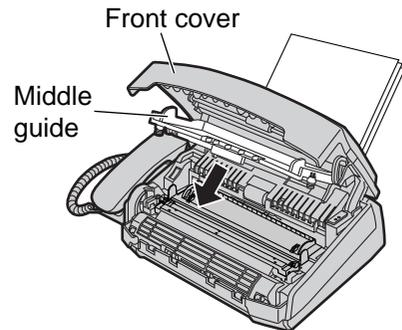
**4** Clean the document feeder rollers with a cloth moistened with isopropyl rubbing alcohol, and let all parts dry thoroughly.
