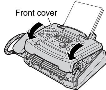
**4** Remove the recording paper. Straighten and reinsert it into the recording paper entrance.
