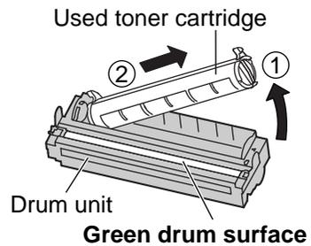
**6** If you replace the drum unit at the same time, remove the new drum unit from the protection bag. Remove the protection bar from the drum unit.
