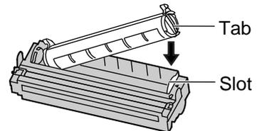
**8a** Hold right side of the toner cartridge under the lip on the drum unit and...
