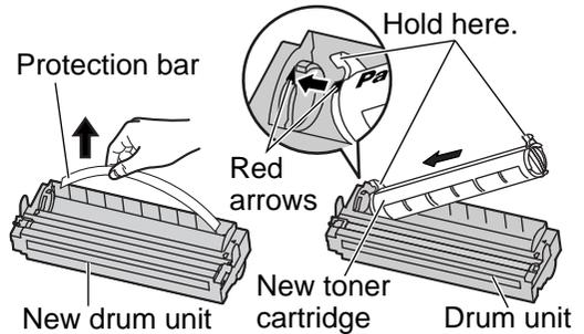
**7** Slide the tab of the toner cartridge into the slot of the drum unit.
